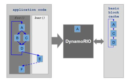
Figure 2.8: DYNAMORIO dynamic binary instrumentation.
