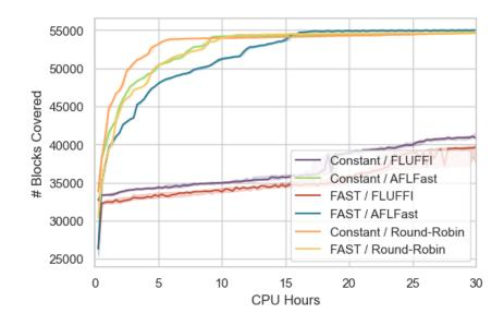
Figure A.6: Median number of basic blocks covered over time for the poppler\_pdf\_fuzzer benchmark with 95% confidence interval.
