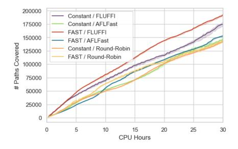
Figure B.5: Median number of paths covered over time for the openh264\_decoder\_fuzzer benchmark with 95% confidence interval.
