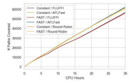
Figure B.3: Median number of paths covered over time for the ffmpeg\_ffmpeg\_demuxer\_fuzzer benchmark with 95% confidence interval.
