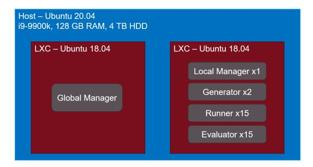
Figure 4.1: Hardware and software configuration for the experiment.
