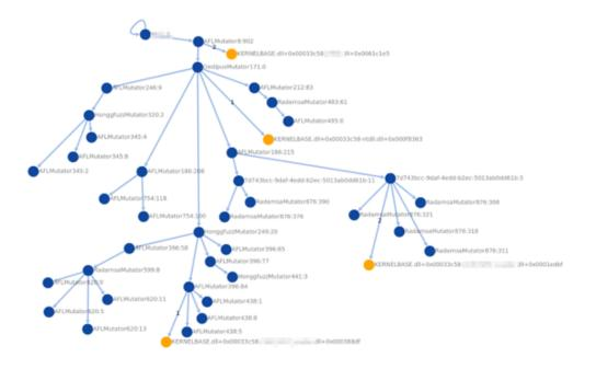
Figure 2.7: FLUFFI mutation tree example [3].
