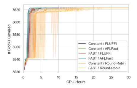
Figure A.7: Median number of basic blocks covered over time for the proj4\_standard\_fuzzer benchmark with 95% confidence interval.
