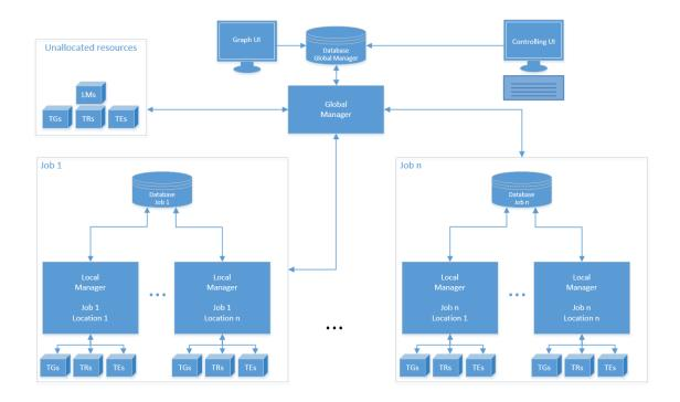
Figure 2.5: FLUFFI global architecture [14].
