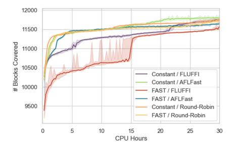
Figure A.5: Median number of basic blocks covered over time for the openh264\_decoder\_fuzzer benchmark with 95% confidence interval.
