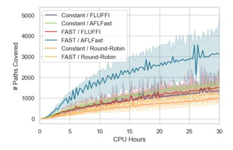
Figure B.7: Median number of paths covered over time for the proj4\_standard\_fuzzer benchmark with 95% confidence interval.
