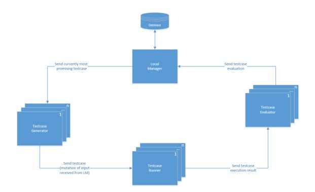
Figure 2.6: FLUFFI local architecture (note: the terms seed and testcase are used interchangeably) [14].
