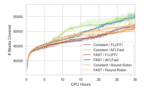
Figure A.3: Median number of basic blocks covered over time for the ffmpeg\_ffmpeg\_demuxer\_fuzzer benchmark with 95% confidence interval.
