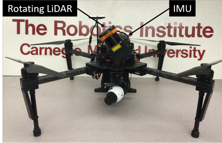
Figure 3.4: The customized robot platform with on board computation and sensing system (rotating laser scanner and IMU). The front camera is for inspection thus is not used for state estimation.
