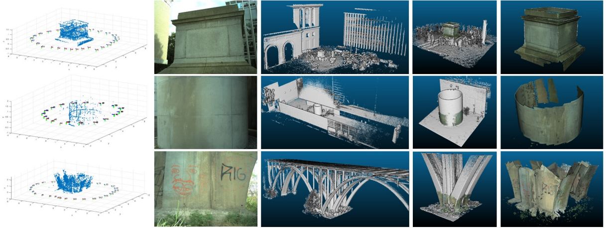
Figure 5.8: From top to bottom, the results of three tests are visualized: a squared pillar (top), a cylinder pillar (middle) and a bridge pillar (bottom). From left to right, we visualize the camera poses and landmarks (blue points), a sample of the image data, complete LiDAR point cloud, overlaid LiDAR and stereo point cloud, dense stereo point cloud.
