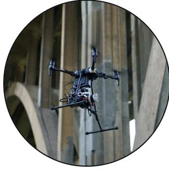
Phase 1: Data Collection UAV collects data autonomously while scanning the structure
