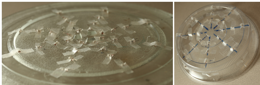
Figure 3.4: A turntable with 32 neon lights (left) and a plate cover with 32 neon lights (right).
