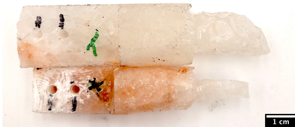
Figure 6.13. Photograph of salt rods after dissolution into deionized H 2 O
