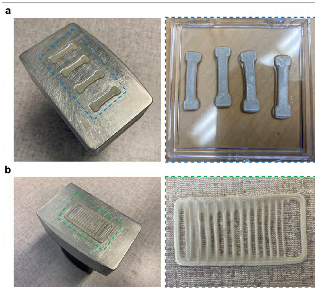
Figure E.1: Printability of UV-curable conductive hydrogel composite using Asiga printer. a , Dogbone shapes. b , Resolution test. The traces' widths are starting at 1.4 mm (left) and decreasing to 0.1 mm (right) by 0.1 mm.
