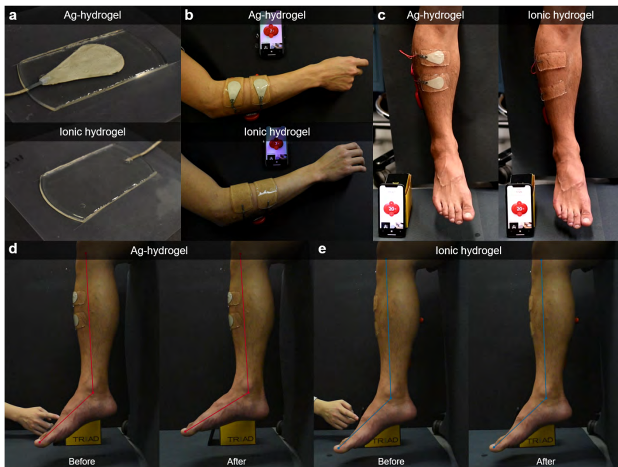
Figure 3.15: Neuromuscular electrical stimulation electrodes. a , The NMES electrodes made of the electrically conductive Ag-hydrogel (top) and ionically conductive PAAM-alginate hydrogel (bottom). b , The electrodes are placed on posterior of the forearm: Ag-hydrogel (top) and ionic hydrogel (bottom). c , The electrodes are placed on the tibialis anterior muscle: Ag-hydrogel (left) and ionic hydrogel (right). d , The side view of the subject's leg before (left) and after (right) electrical signal delivered by the electrodes made of the Ag-hydrogel. The red lines were used to track the change in dorsiflexion angle. e , The side view of the subject's leg before (left) and after (right) electrical signal delivered by the electrodes made of the ionic hydrogel. The blue lines were used to track the change in dorsiflexion angle.
