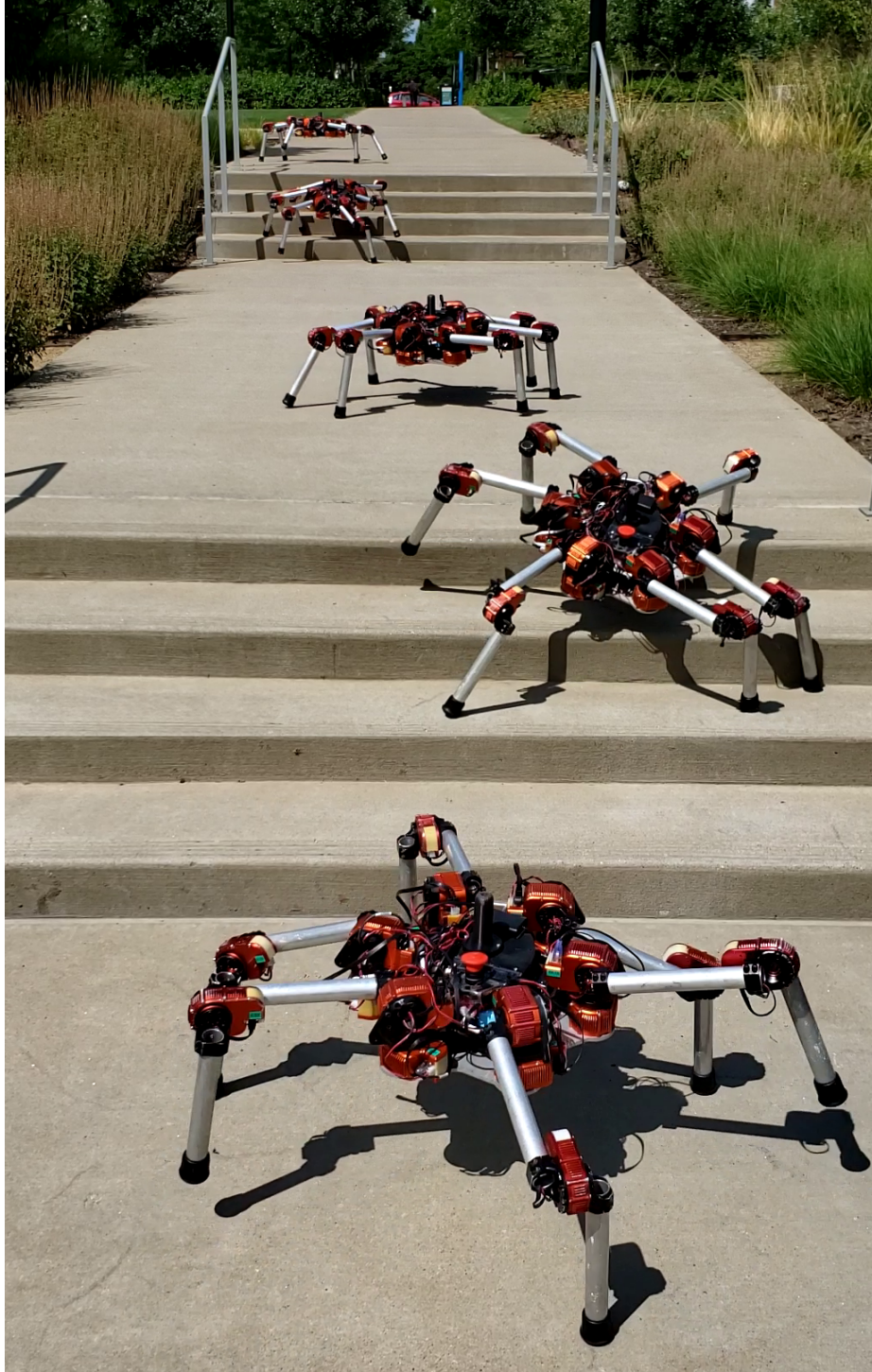
Figure 4-5: A time-lapse of a hexapod climbing up stairs using the onboard vision system and modular visual-motor policy. The steps in the stairs shown here are 14 cm high, comparable to the height of the robot body at its nominal resting stance.
