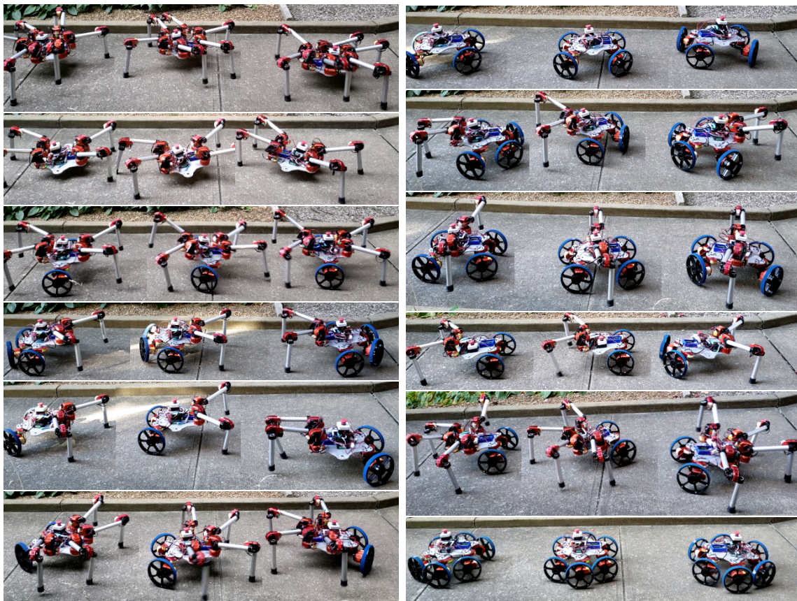
Figure 3-10: Timelapses of the twelve modular designs controlled with the learned policy. The robots were teleoperated with a joystick demonstrating forward and turn-in-place locomotion on a sidewalk.
