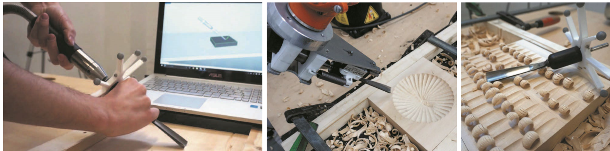
Figure 11. Data collection apparatus, training samples, and execution of learned motions, image from (Brugnaro and Hanna 2017).
