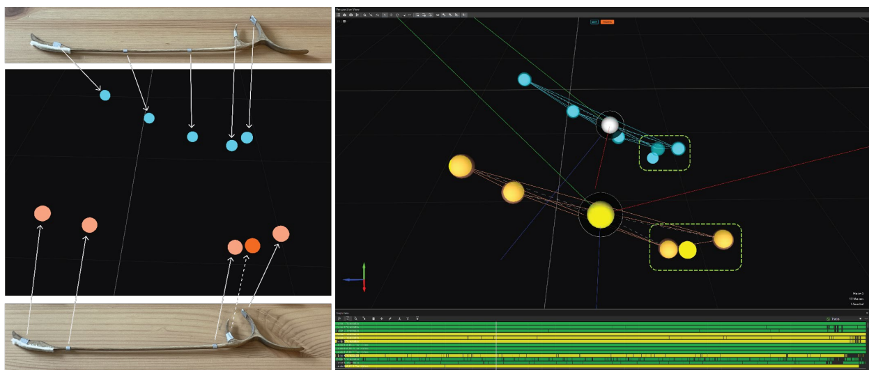
Figure 64. Flat retro-reflective trackers on the mezarab (left), corresponding registered ones in the Motive app (right).
