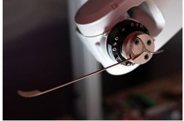
Figure 82. Mezrab holder, detailed view (left), installed on the robot (right).
