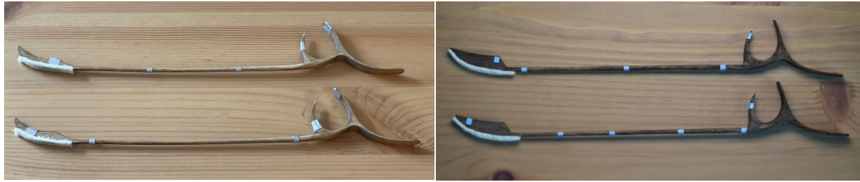
Figure 65. Early retro-reflective marker arrangement (left) and revised version (right), notice the slight differences between the marker arrangement on each pair of mezrabs.
